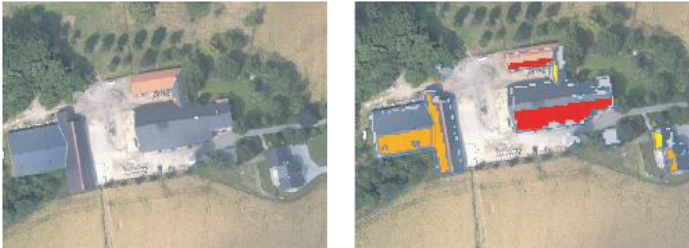
Figure 18.13 | Example of assessing local renewable potentials: roof area (left panel) and suitable roof-area identification for solar PV applications (right panel) for the city of Osnabrück, Germany. Red: roof area well suited for PV; orange: suitable; yellow, only conditional suitability for PV applications; grey: shadowed roof area (unsuitable). Source: modified from Ludwig et al., 2008.
