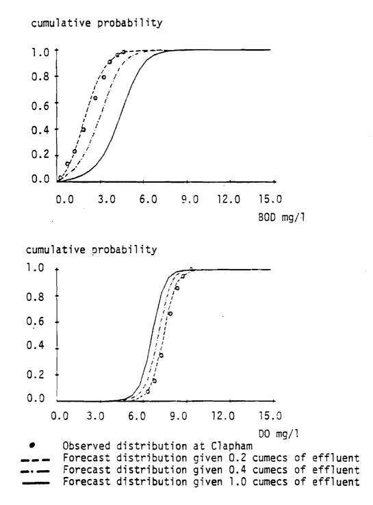
Figure 5. Distributions of DO and BOD at Clapham obtained from the Monte Carlo Simulation Study
