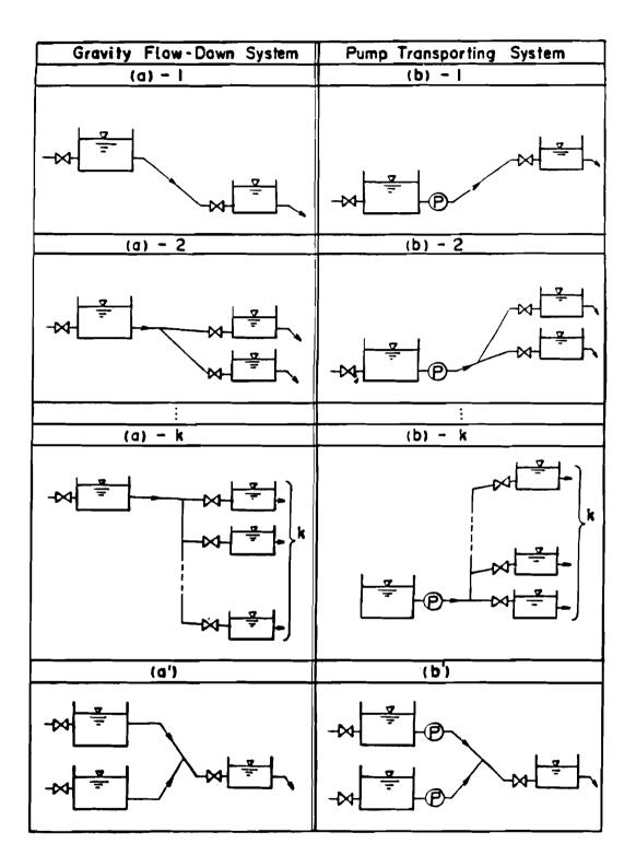
Figure 3. Calculation Modules for a Water Transportation System
