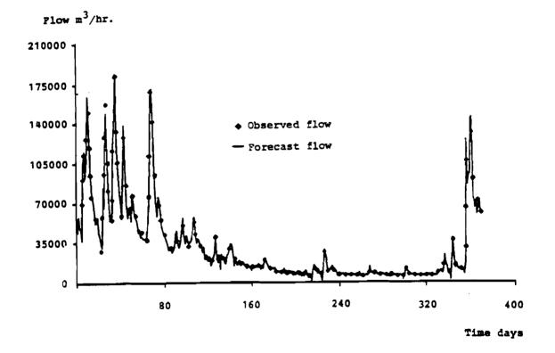
Figure 3. Simulated, Observed and Residual Flows on the Bedford Ouse over 1972
