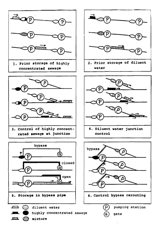
Figure 1. Diagrams of the Mixing and Dilution Control Methods
