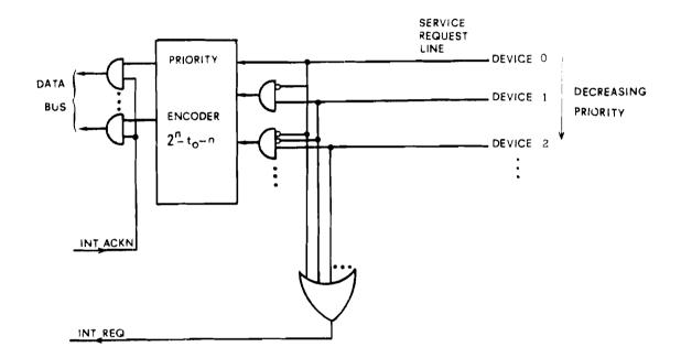
Figure 5. A simple way to create priorities among a number of interrupt lines. Interrupt philosophy is preferred when peripheral servicing is assigned a high preference, otherwise flag bit testing may represent a simple way of servicing a great number of peripherals.
