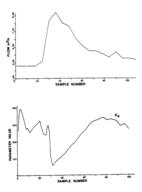
Figure 8. Recursive Estimate of Ammonia Decay Coefficient and Measured Flow at Tempsford
