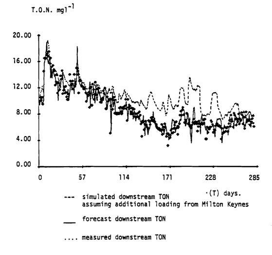
Figure 4. Simulated and Observed Daily TON Concentrations on the Bedford Ouse during 1974
