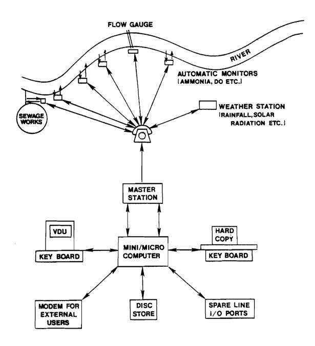
Figure 6. Monitoring, Telemetry and mini/micro Computing System Operational Management
