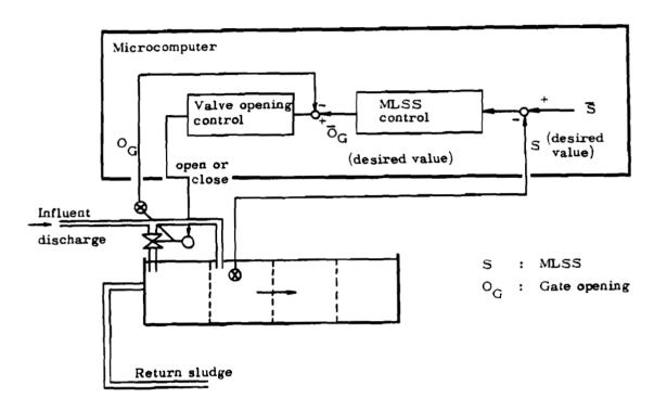
Figure 7. Block diagram of dynamic sludge reserving system
