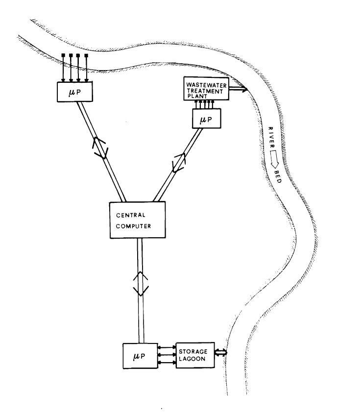
Figure 1. A scheme for a water quality monitoring network, showing peripheral stations (surveillance and/or control-oriented),the central computer and the digital communication links.
