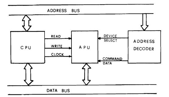
Figure 8a. System wiring to interconnect APU with the rest of the microcomputer system. Both system buses are involved in addition to a few control lines.
