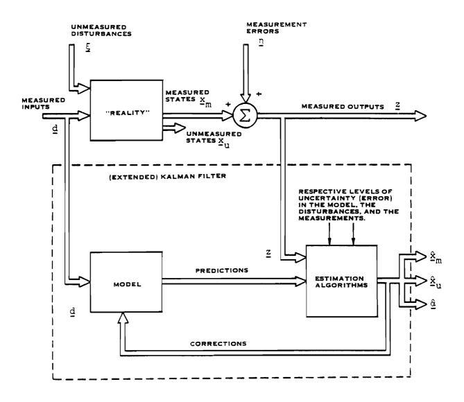
Figure 2. The (extended) Kalman Filter, an algorithm for estimation and forecasting;  $\frac{\dot{x}}{m}$ ,  $\frac{\dot{x}}{u}$ , and  $\frac{\hat{\alpha}}{a}$  are respectively estimates of the measured state variables, the unmeasured state variables and the model parameters.
