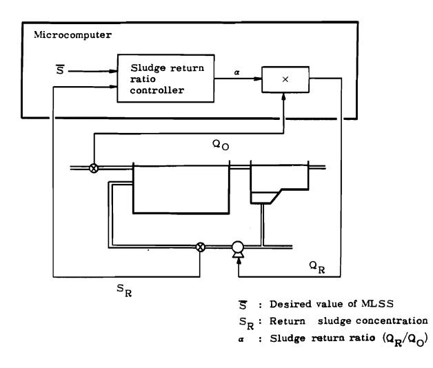
Figure 6. Block diagram for MLSS controller
