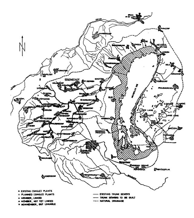
Figure 2. Drainage Basin of Neusiedlersee with Location of Wastewater Treatment Plants.
