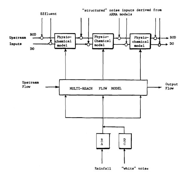
Figure 1. Interaction between Hydrological and Water Quality Models
