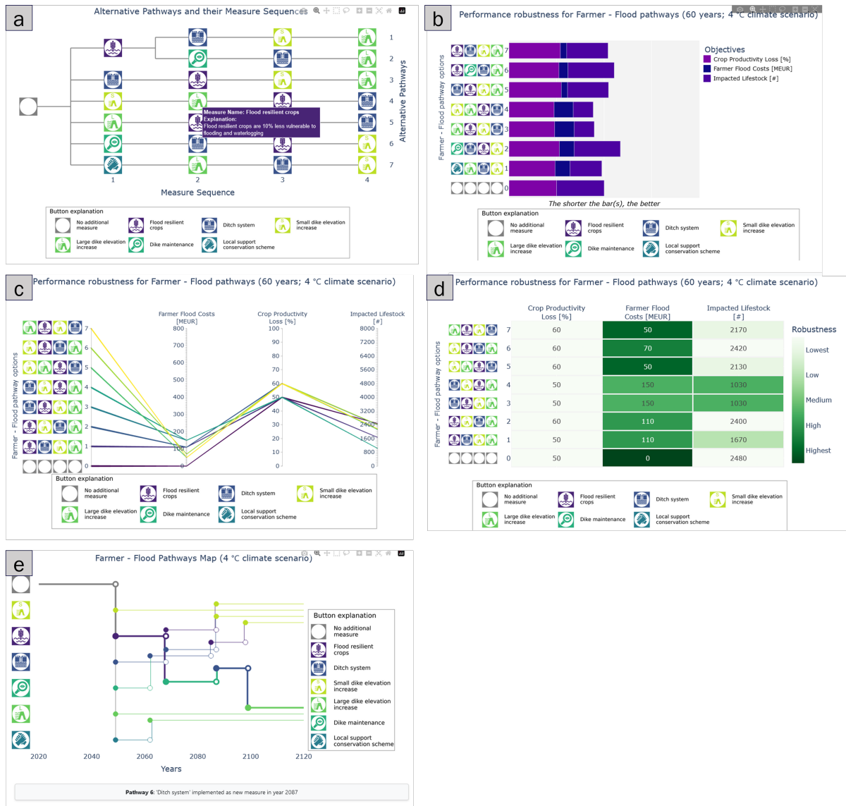
Figure 2. Set of visualisation types for pathways analysis. visualisation of pathways options by means of DT (a). Interactive components offer information on demand. SBC (b), PCP (c) and HM (d) to explore pathways performance across multiple objectives for different pathways options. Pathways map to investigate the timing of decision-making (e).
