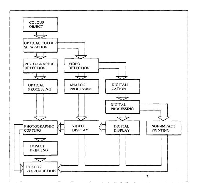
Fig. 3 Alternatives of the production of multiple copies in imaging technologies.
