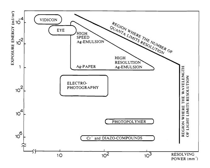
Fig. 5 The requirement of exposure energy and the corresponding resolving power for some detection techniques /6,11,18,26,32,37/.
