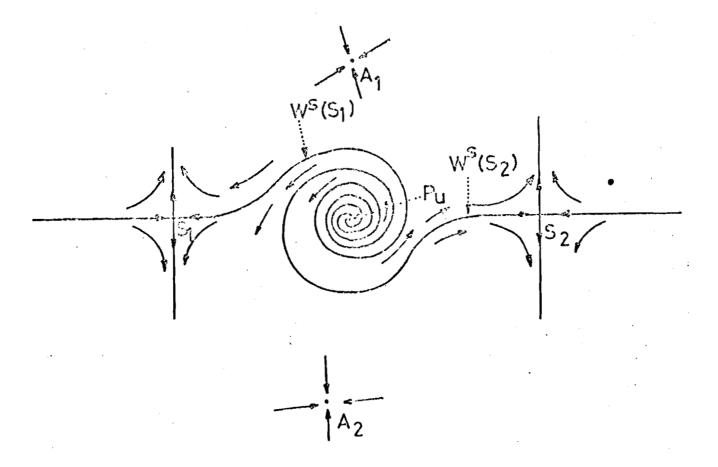
$A_1$ ,  $A_2$  are attractors,  $S_1$  and  $S_2$  saddles and  $P_u$  an instable fixed point. The separatrices  $W^S(S_1)$  and  $W^S(S_2)$  wrap around  $P_u$  infinitely often and so the basins of  $A_1$  and  $A_2$  are completely intermeshed.
