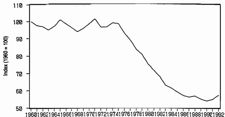
Figure 9. Trends in unit energy consumption in Japanese manufacturing industry, 1960–1992. Index: 1960 = 100. Unit energy consumption: energy consumption per IIP (production weight).
