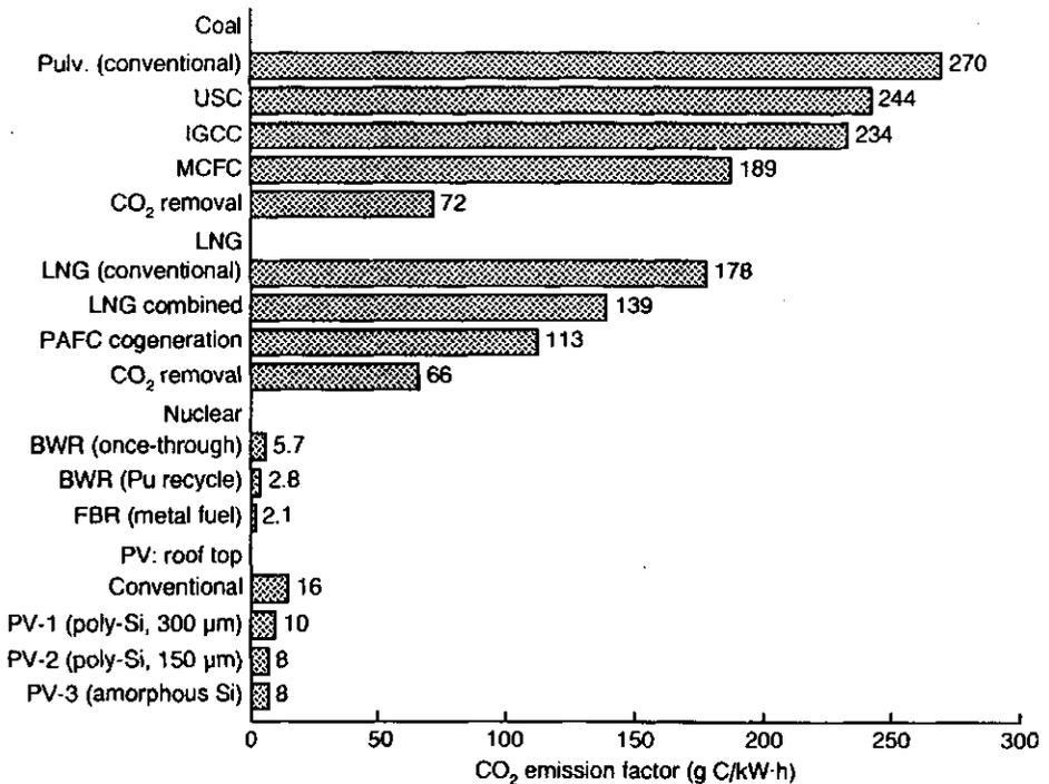
FIG. 6. CO<sub>2</sub> emission factor of advanced electricity supply systems.
