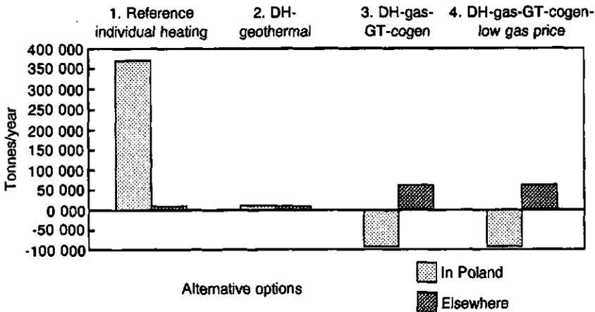
FIG. 4. Poland (Zakopane): GHG emissions of different supply alternatives (results of the EM scenario calculation).
