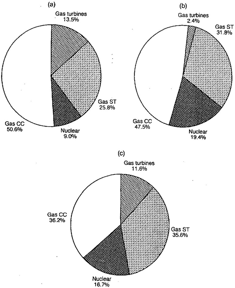
FIG. 7. Structure of new capacities for the reference case and the sensitivity cases (in per cent of the total installed capacity of new units entering the system by the year 2015). (a) Reference case, (b) low demand case, (c) high demand case.
