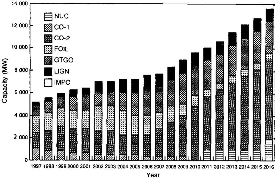
FIG. 23. Total installed capacity in a thermal system — optimization mode.
