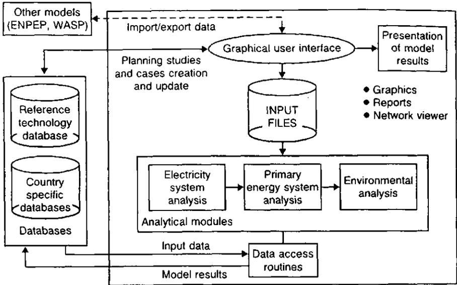
FIG. 19. System level analysis.
