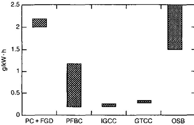
FIG. 10. Emissions of NO<sub>x</sub> — power plant level.
