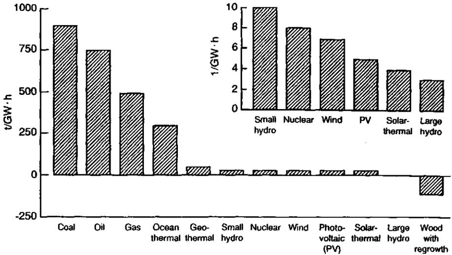
FIG. 7. Carbon dioxide emissions from different electricity generating technologies [27].
