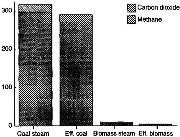
FIG. 5. Sri Lanka electricity fuel chains: global warming potential (t CO<sub>2</sub> equivalent per 1000 GJ; IPCC 100 year integration, see Ref. [5]).
