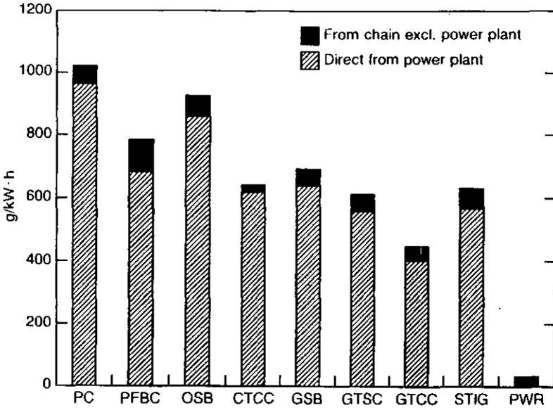
FIG. 14. Emissions of CO<sub>2</sub> — full chain.
