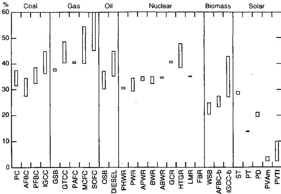
FIG. 7. Preliminary comparison of generating efficiency for RTDB technologies (see Table I).
