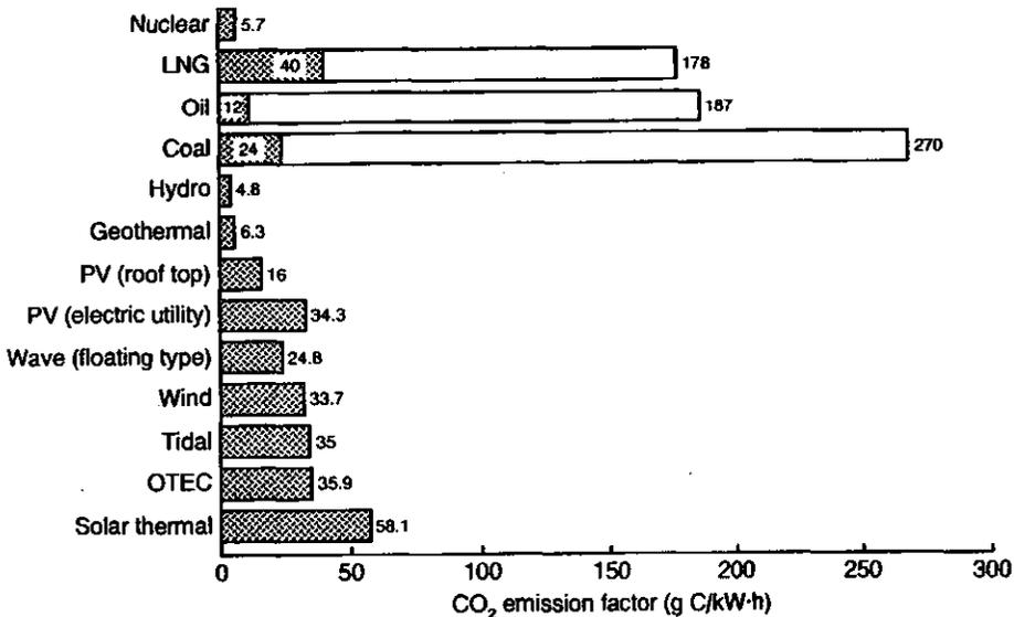
FIG. 5. Greenhouse gas emission factor of different electricity generation systems.
