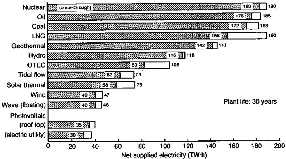
FIG. 3. Net electricity supplied by electricity generation systems (1000 MW).
