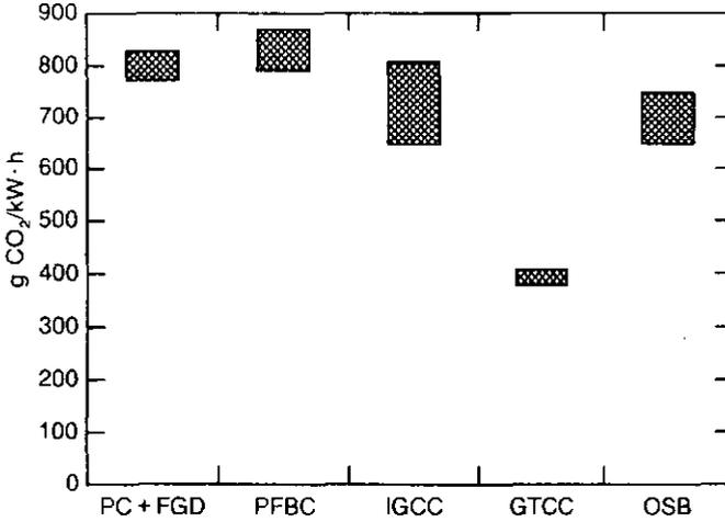
FIG. 9. Emissions of CO<sub>2</sub> — power plant level.
