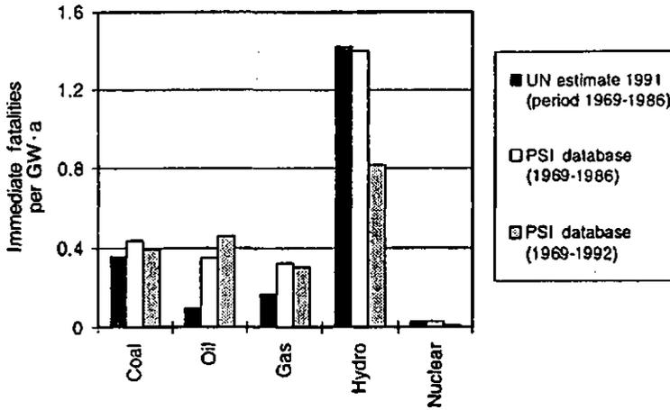
FIG. 9. Comparison of records of energy related severe accidents: immediate fatality rate per unit of energy (source: PSI database, June 1995).
