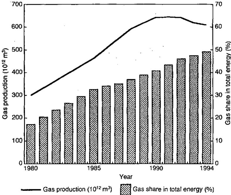
FIG. 2. Production of natural gas and its share in the total energy balance of Russia.
