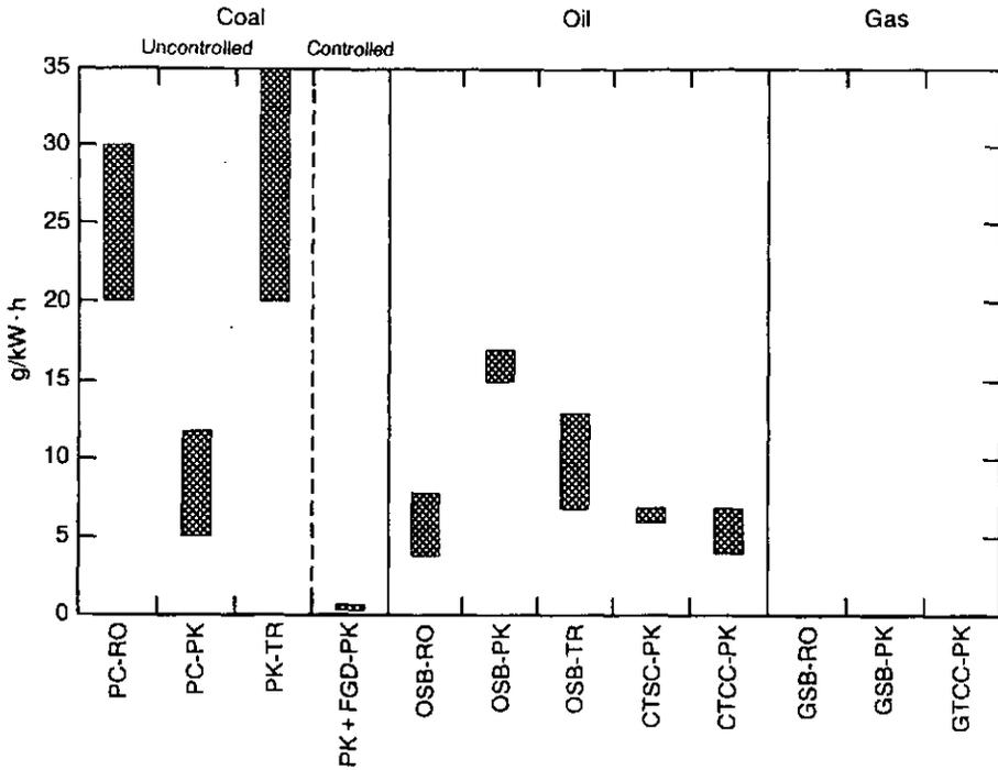
FIG. 11. Emissions of  $SO_x$  — power plant level.
