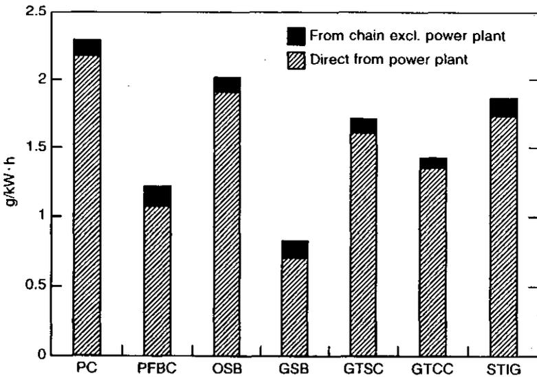
FIG. 15. Emissions of NO<sub>x</sub> — full chain.
