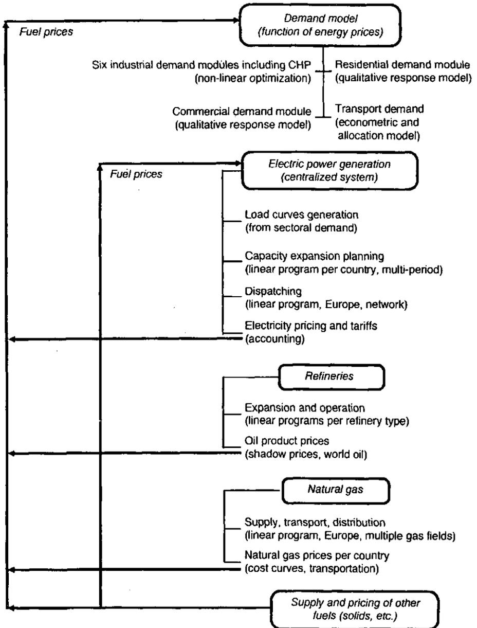
FIG. 7. Schematic of the general model.
