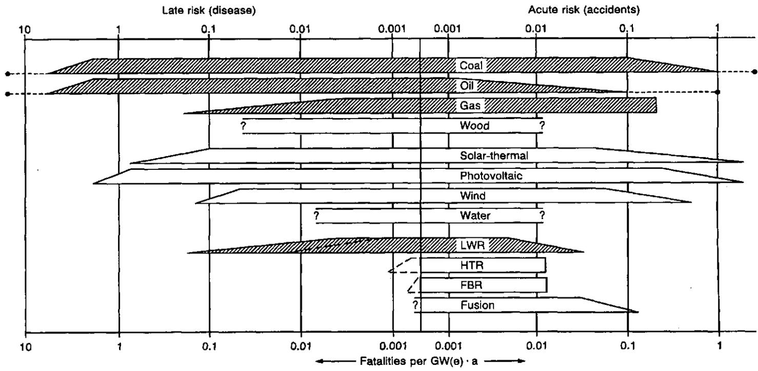
FIG. 6. Public mortality risks due to electricity production for all steps of the fuel cycle, without severe accidents [23, 24].
