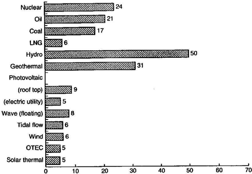
FIG. 2. Energy ratio of electricity generation systems (without T&D).
