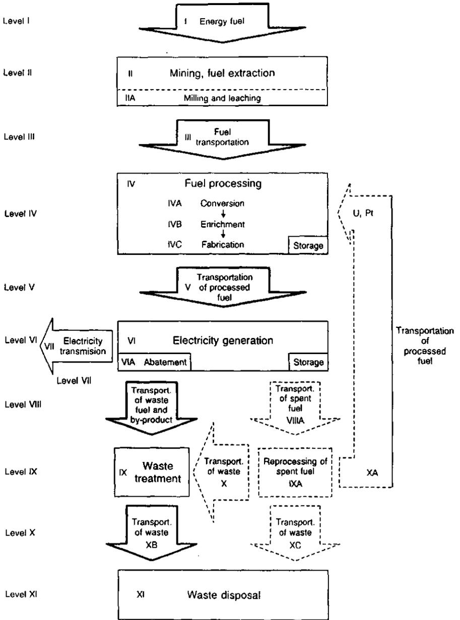
FIG. 4. Graphical representation of a generalized fuel chain [3].
