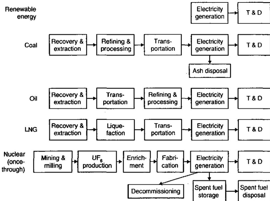
FIG. 1. Scope of fuel chain processes of electricity supply systems.
