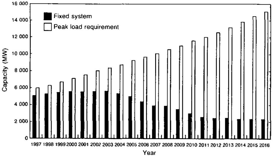
FIG. 21. Installed capacity in a fixed system and capacity required for peak load.
