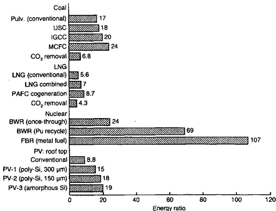
FIG. 4. Energy ratio of advanced electricity supply systems.
