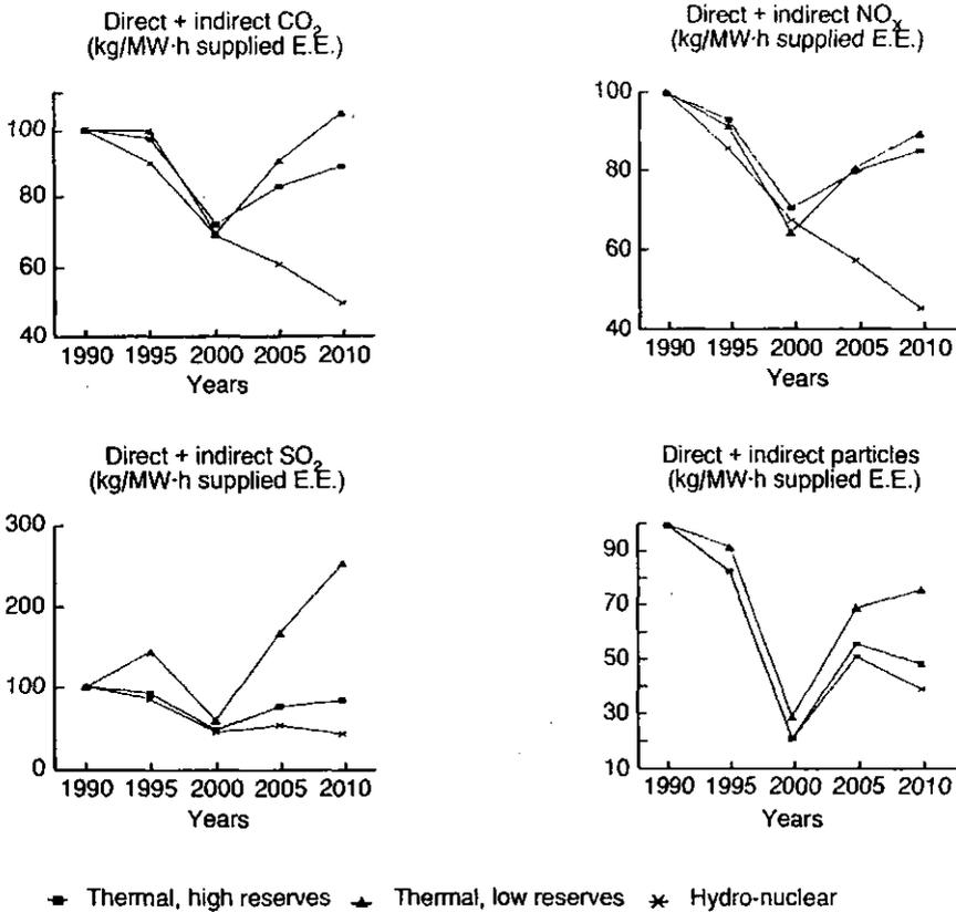
FIG. 5. Evolution of direct and indirect emissions (1990 basis).
