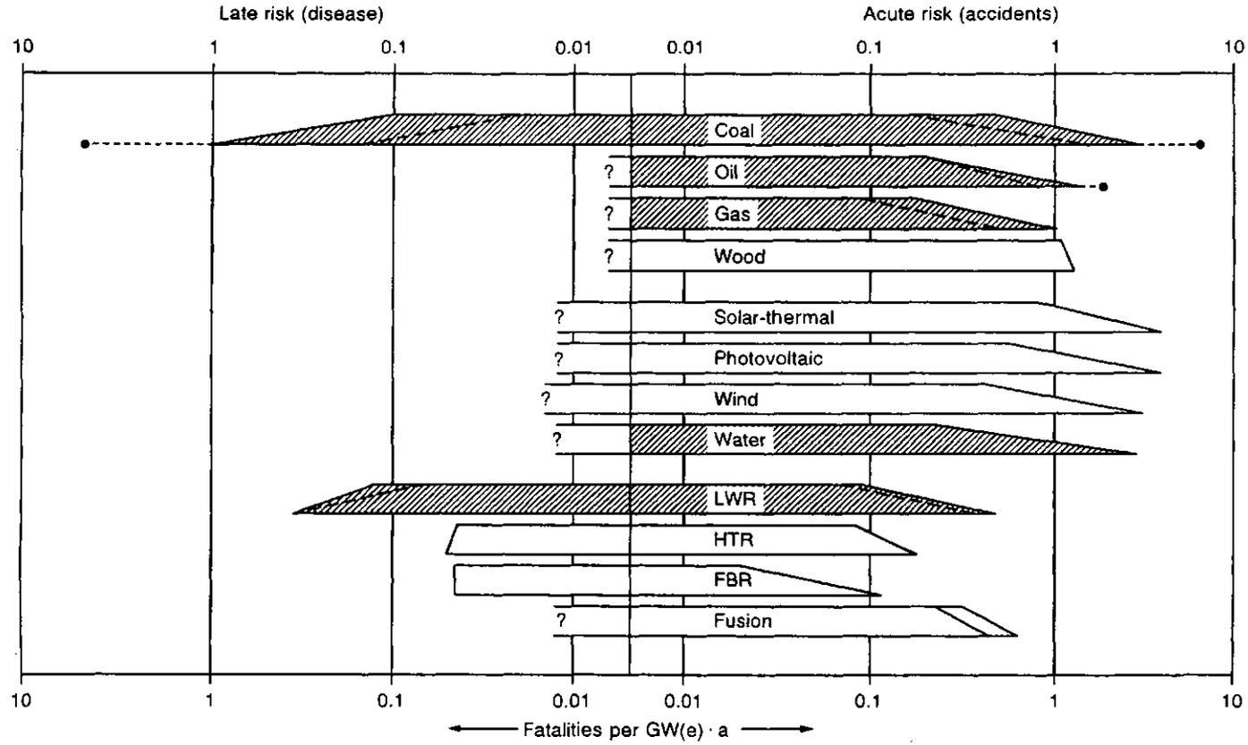
FIG. 5. Occupational mortality risks due to electricity production for all steps of the fuel cycle, without severe accidents [23, 24].
