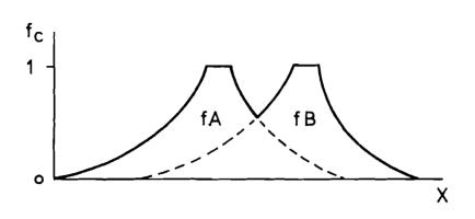
Fig. 3.4 The membership function associated with the union C of A and B
