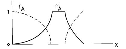
Fig. 3.3 The membership functions  $f_A$  and  $f_{A'}$ , associated with the fuzzy set A and its complement A', respectively
