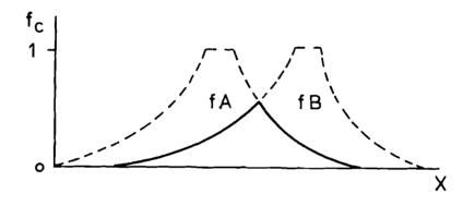
Fig. 3.5 The membership function associated with the intersection C of A and B
