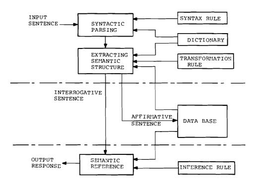
Figure 2. Functional diagram of a QAS.
