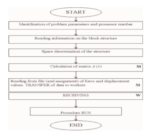
**Figure 7.** Scheme of parallelization of the block model. Notation: operations carried out only by master are marked by "M", only by workers – by "W"
