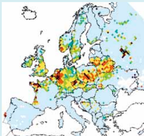
FIGURE 8.6 Percentage of ecosystems area for which acid deposition above sustainable critical loads is calculated for 2020 (assuming full implementation of current EU air quality legislation). Lefthand map: for a business-as-usual baseline energy projection that results in 3% higher GHG emissions compared to 1990; righthand map: for an energy scenario with GHG emissions 20% below the 1990 level.
